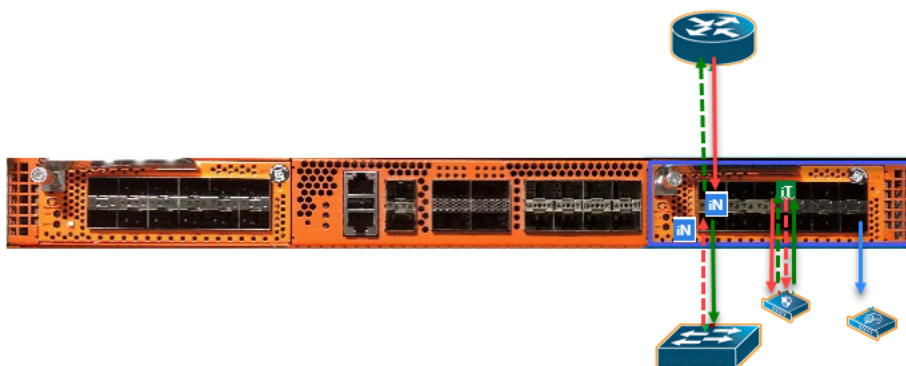
Figure 61 Logical Bypass Without Bypass Combo Module
