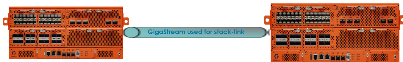
Figure 4 Daisy-Chain Configuration using GigaStream for Stack-link
